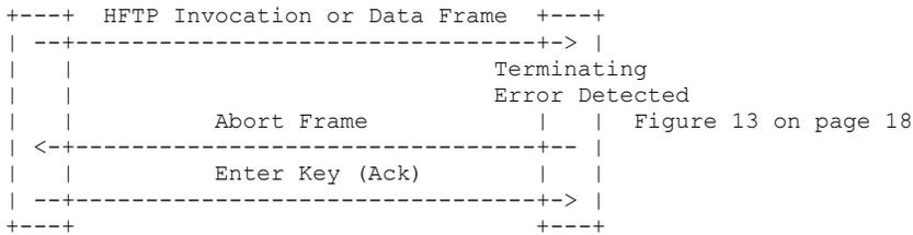
Figure 10. Terminating Error Sequence (CUT) Initiated by the Host
