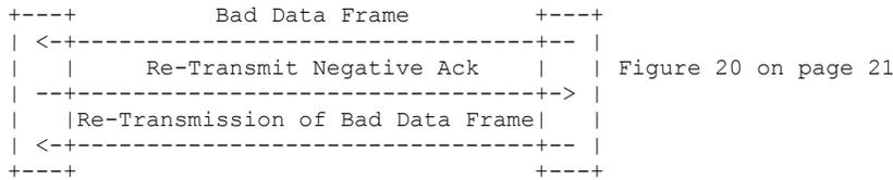
Figure 7. Data Error Sequence (CUT) Initiated by PC
