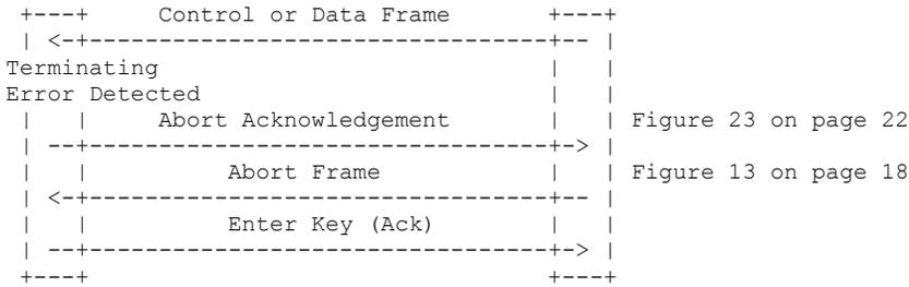
Figure 9. Terminating Error Sequence (CUT) Initiated in PC
