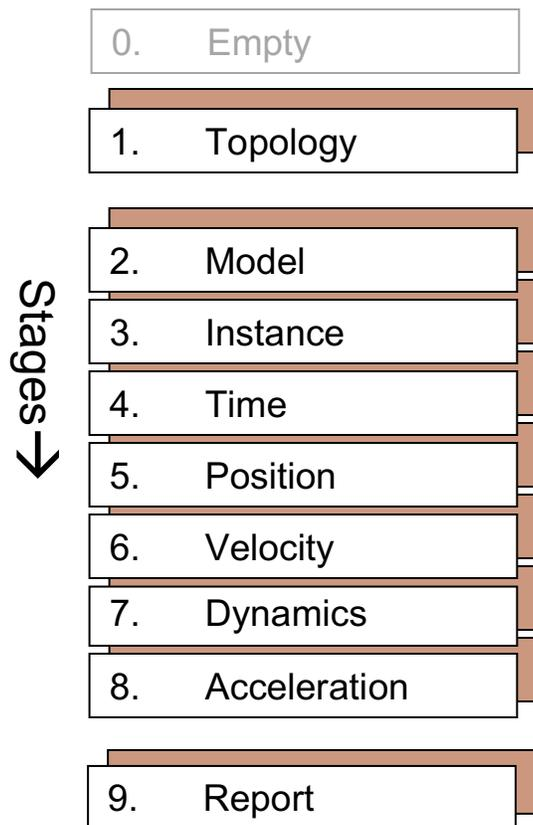
**Figure 4.** The organization of a computation into ordered stages. When a State is realized to a given stage, the cache information for that stage (shown in brown) is calculated and filled in. A change to a state variable at a given stage invalidates cache information at that stage and higher.
