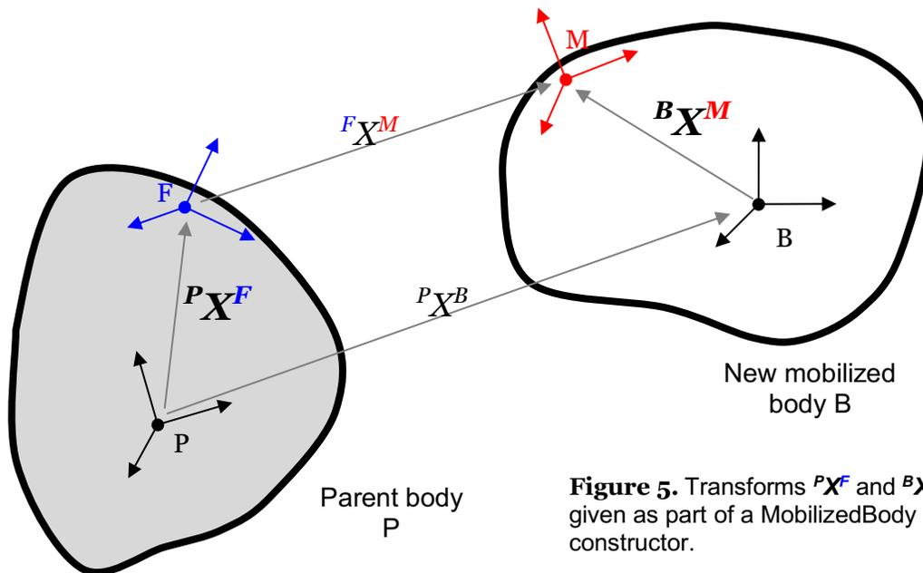
**Figure 5.** Transforms  $PX^F$  and  $BX^M$  are given as part of a MobilizedBody constructor.
